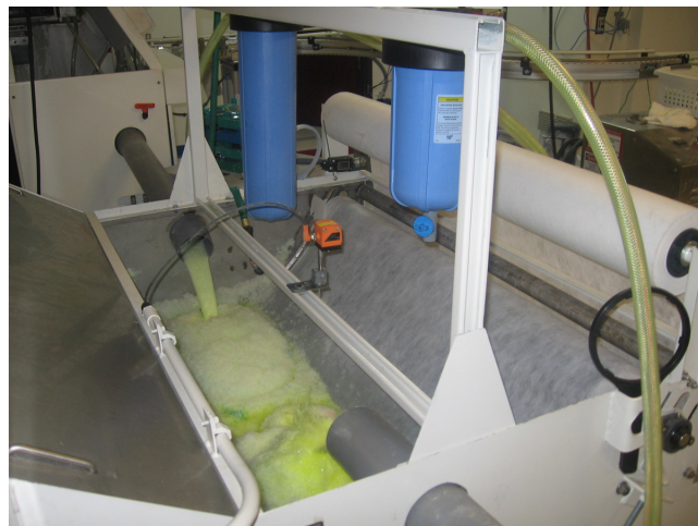
Figure 2 Optical lens generation coolant discharge for two machines into the bed of the filter
