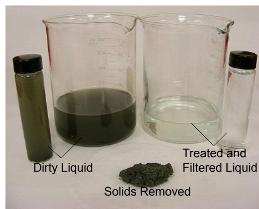
Figure 4 Waste water, Floc, Filtrate, Filtered Solids
