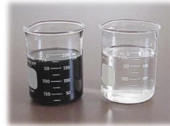
Figure 5 Boiler Fly Ash Water (left), Clean Filtrate (right)
