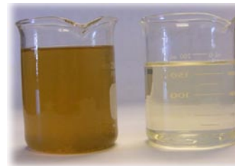
PVC Extrusion Water (left), Clean Filtrate (right)
