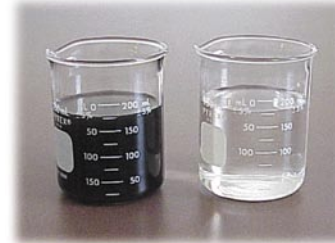
Boiler Fly Ash Water (left), Clean Filtrate (right)
