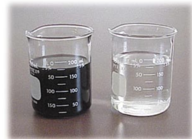
Figure 4 Dirty Caster Water (left), Clean Filtrate (right)
