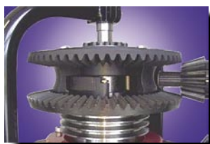
◀ Patented Ring and Pinion Gear Bowl Cleaning Mechanism
