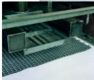
Patented labyrinth side seal design.
