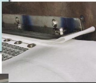
Low velocity inlet distribution header.
