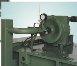
Low velocity inlet distribution header.
