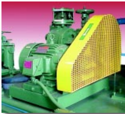
Belt Driven Bottoms Pump designed for high vacuum pump suction operation.
