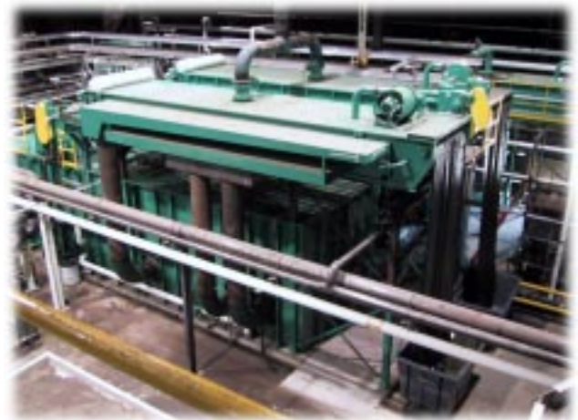
▲ Typical Cold Rolling Filtration System with Flatbed Vacuum Filters and Magnetic Separator Clarifiers.
