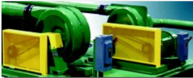
High volume/low differential vacuum producer for ramp, and low volume/high differential vacuum producer for liquid pool.
