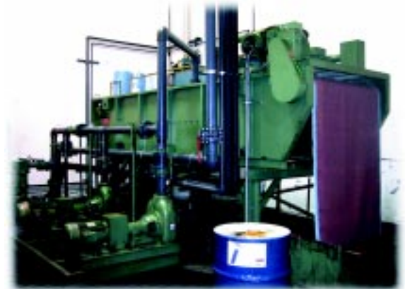
Typical Centralized Filtration System ▲ For Copper Wire Drawing.
