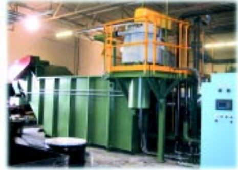
Aluminum Wire Drawing Filtration System. ▼
